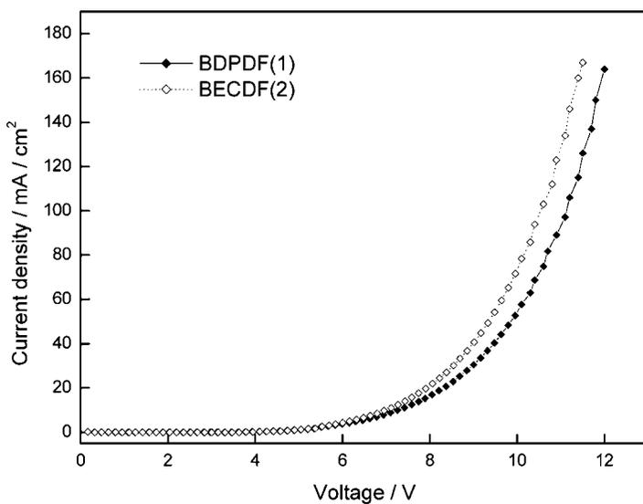
**FIGURE 3** Current-voltage (I-V) characteristics of undoped EL devices.
