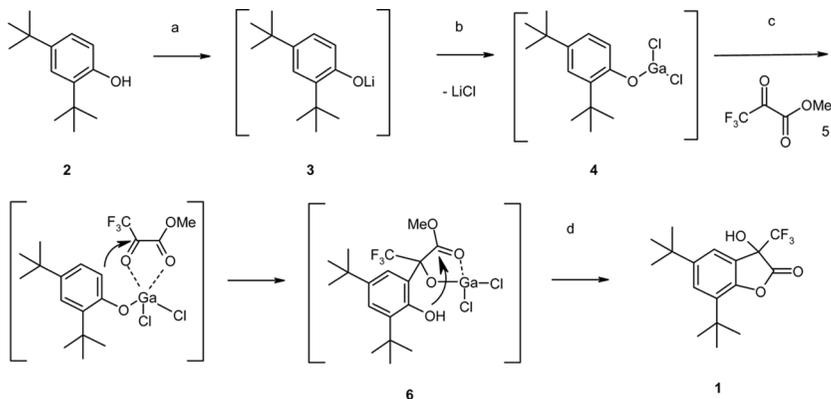
**Scheme 1.** (a) n-Bu Li (1 eq), THF,  $-70$  to  $20^{\circ}\text{C}$ , distill off THF; (b) GaCl<sub>3</sub> (1 eq), DCE,  $-10$  to  $80^{\circ}\text{C}$ , 15 min; (c) CF<sub>3</sub>COCO<sub>2</sub>Me (1 eq), DCE,  $0$ – $20^{\circ}\text{C}$ ; (d) DCE,  $28$ – $80^{\circ}\text{C}$ .
