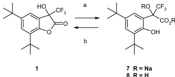
**Scheme 2.** (a) 1 N NaOH (2 eq), dioxane, 0–20 °C, 16 h; (b) 1 N HCl, AcOEt, 0 °C, upon extraction.
