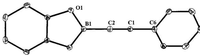
Figure 2. Molecular structure of **5a** in the solid state; hydrogen atoms are omitted for clarity; selected bond lengths [Å] and bond angles [°]: C1–C2 1.196(5), C1–C6 1.447(5), B1–C2 1.513(5), B1–O1 1.383(15), C1–C2–C6 180.0, C1–C2–B1 180.0
