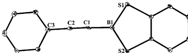
Figure 3. Molecular structure of **6a** in the solid state; hydrogen atoms are omitted for clarity; selected bond lengths [Å] and bond angles [°]: C1–C2 1.207 (8), C2–C3 1.423(7), B1–C1 1.521(8), B1–S1 1.796(6), C1–C2–C3 178.5(5), C2–C1–B1 177.6(5)
