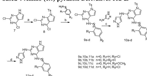
Conditions and reagents: (a), TsCl, Et<sub>3</sub>N, DMAP, CH<sub>2</sub>Cl<sub>2</sub>, r.t. 5 h. (b) DIPEA, *n*-BuOH, 100 °C, overnight. (c) TFA, *n*-BuOH, 120 °C, 1 h, microwave (MW irradiation). (d) Cs<sub>2</sub>CO<sub>3</sub>, H<sub>2</sub>O:CH<sub>3</sub>OH:dioxane=1:3:3 (V/V/V), 80 °C, 6 h.
