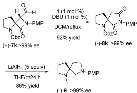
ment of (-)-**8k** with 5 equiv of LiAlH<sub>4</sub> in THF led to a spiro bicyclic diamine (-)-**9**. It should be noted the spiro bicyclic diamine structures exist extensively in pharmaceutical compounds,<sup>17</sup> and the current methodology provides a facile access to their optically pure form.
