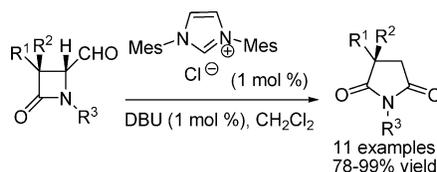
**N**-heterocyclic carbene (NHC) has been employed as an efficient catalyst for ring expansion of 4-formyl- $\beta$ -lactams, allowing the facile synthesis of succinimide derivatives. This organocatalytic process features readily availability of the catalyst, low catalyst loading, and mild reaction conditions.
