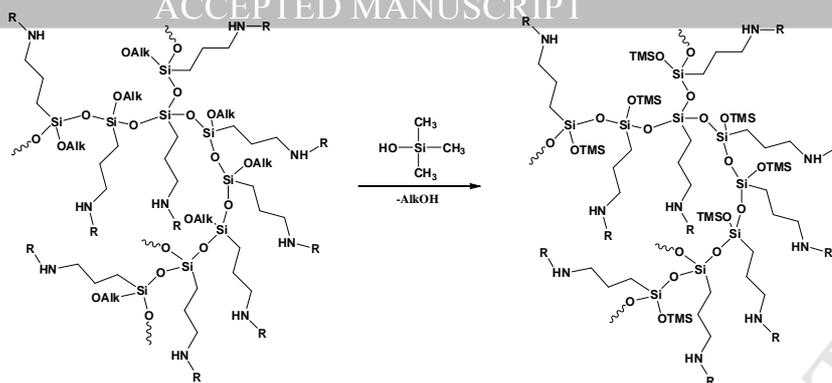
**Scheme 7.** Synthetic scheme of termination of hyperbranched polyaminopropylalkoxysilanes with trimethylsilanol.
