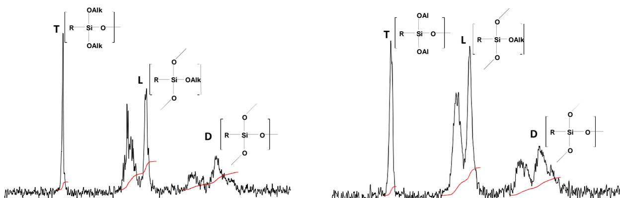
**Figure 6a.**  $^{29}\text{Si}$  NMR spectra of polyaminopropylethoxysilane
