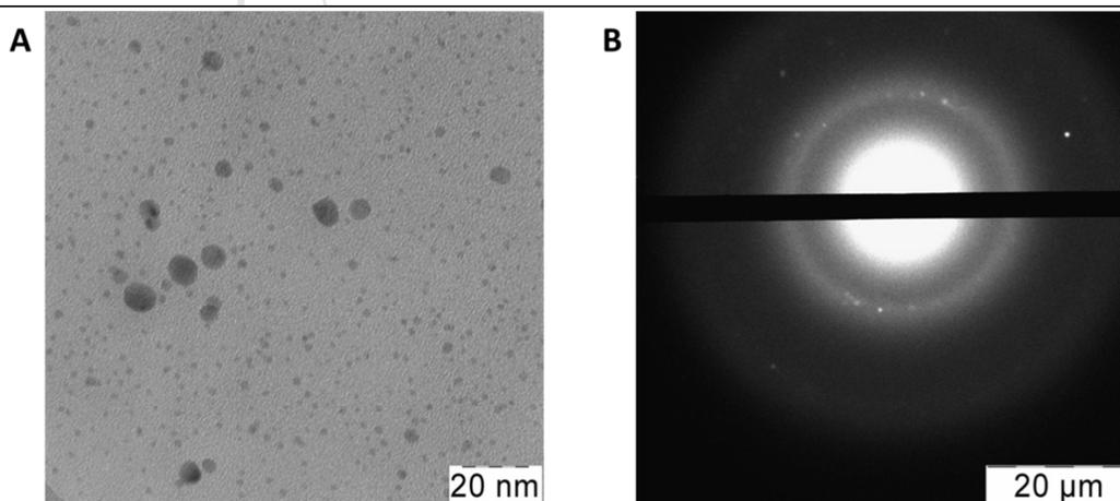
**Figure 11.** TEM image of Ag nanoparticles stabilized with HBPEDAPS matrix (A); electron diffraction ring pattern from a crystalline Ag specimen (B).
