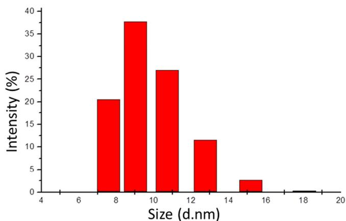
**Figure 10.** Distribution of Ag nanoparticles obtained after irradiation of a solution of the HBPEDAPS matrix and AgBF<sub>4</sub> in methanol, estimated by DLS method.
