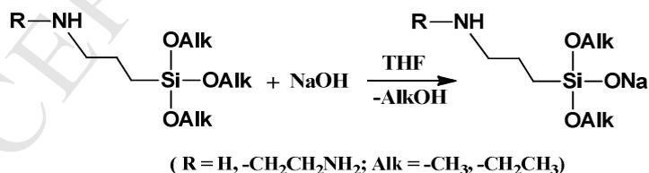
**Scheme 1.** Synthetic scheme for monosodiumoxyaminopropyltrialkoxysilanes
