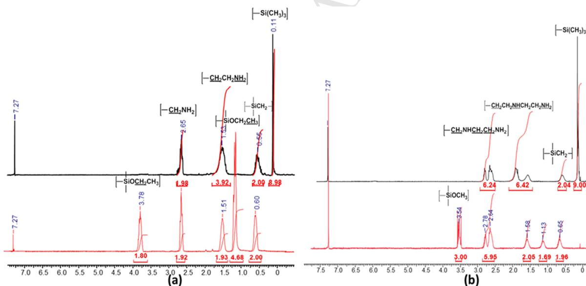
**Figure 7.** <sup>1</sup>H NMR spectra (CDCl<sub>3</sub>) of polyaminopropylethoxysiloxane (a) and polyethylenediaminopropylmethoxysiloxane (b) before (—) and after (—) the termination with trimethylsilanol.
