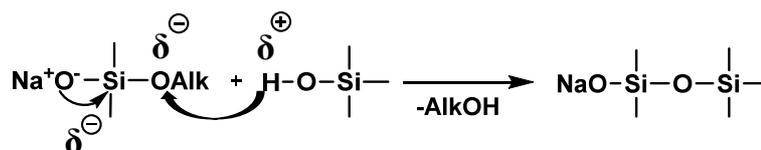
**Scheme 5.** Mechanism of heterofunctional condensation of sodiumoxyalkoxysilane and silanol.
