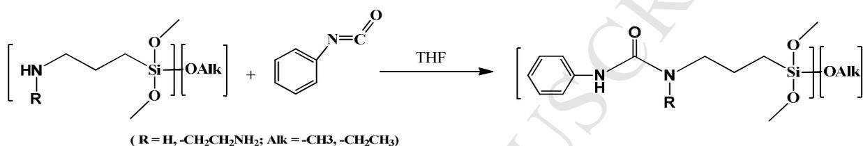
**Scheme 6.** Synthetic scheme of termination of amino groups in hyperbranched polyaminopropylalkoxysiloxane (HBPAPES) with phenyl isocyanate.
