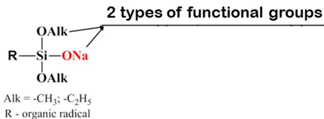
**Figure 4.** Monosodium salts of organotrialkoxysilanes - AB<sub>2</sub>-type monomers
