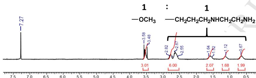
**Figure 5.**  $^1\text{H}$  NMR spectra ( $\text{CDCl}_3$ ) of polyethylenediaminopropylmethoxysilane
