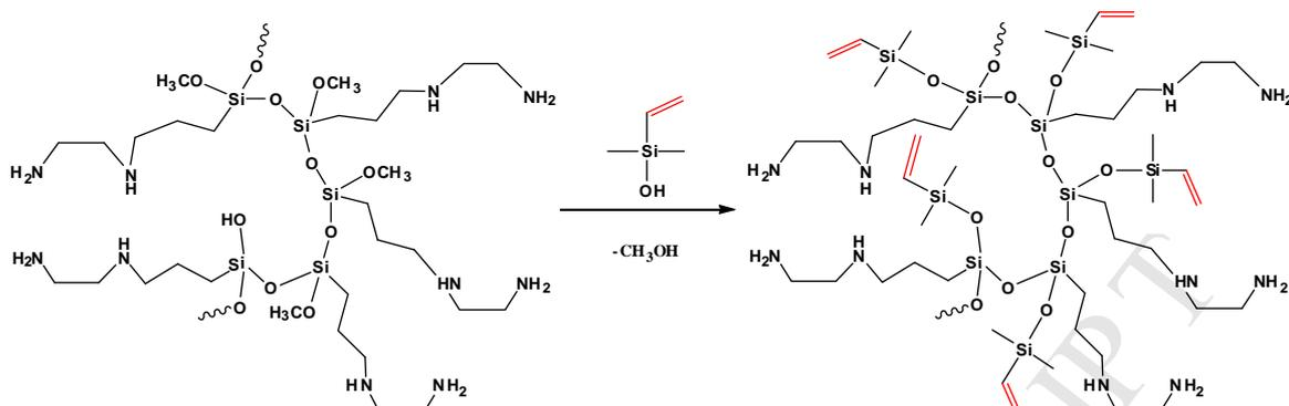
**Scheme 8.** Synthetic scheme of the capping reaction of hyperbranched polyethylenediaminopropylmethoxysilane (HBPEDAPMS) with dimethylvinylsilanol.
