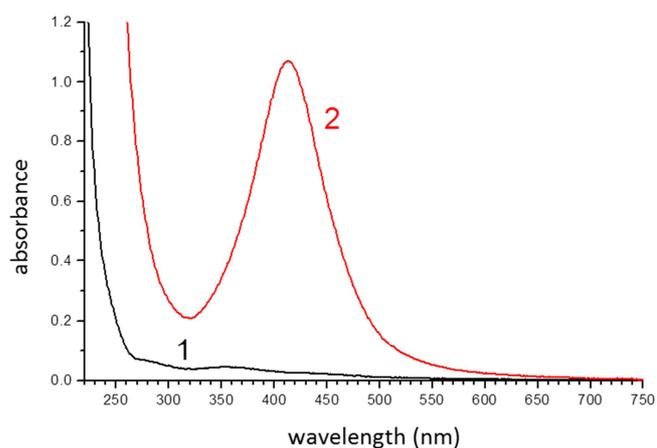
**Figure 9.** Absorption spectra of the HBPEDAPS matrix in methanol (5 mg/ml) (1) and a mixture of the HBPEDAPS matrix and AgBF<sub>4</sub> in methanol after irradiation (2).
