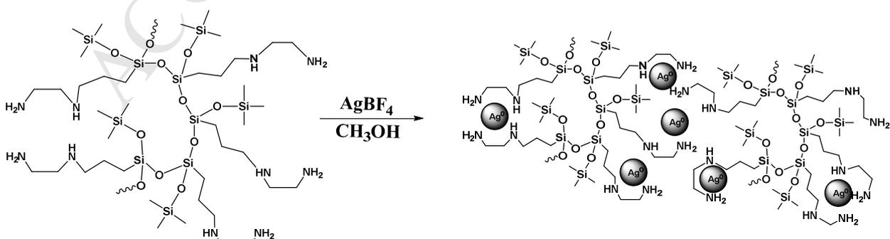
**Scheme 10.** Synthetic scheme of the stabilization of Ag nanoparticles with HBPEDAPS matrix in methanol.
