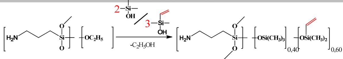
**Scheme 9.** Synthetic scheme of the capping reaction of hyperbranched polyaminopropylethoxysiloxane (HBPAPE) with trimethyl- and dimethylvinylsilanol; synthesis of hyperbranched polyorganosiloxane with two types of terminal groups.
