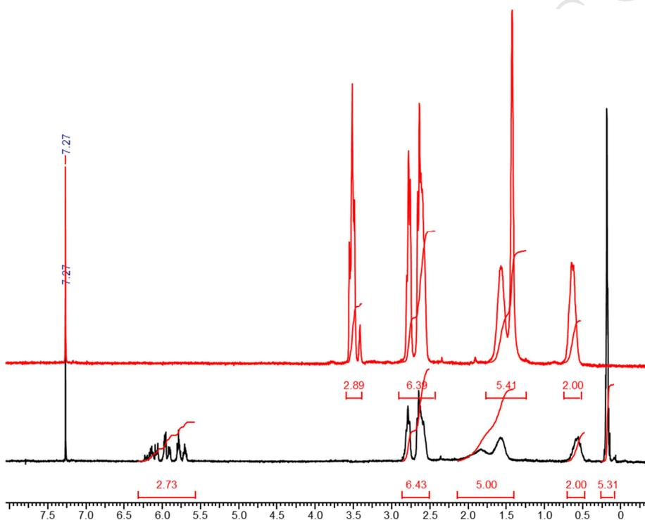
**Figure 8.**  $^1\text{H}$  NMR spectra ( $\text{CDCl}_3$ ) of polyethylenediaminopropylmethoxysilane before (—) and after (—) capping with vinyl dimethylsilanol (from bottom).
