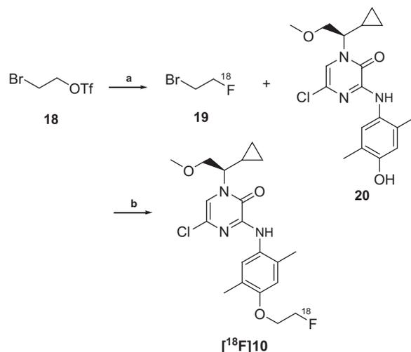
**Scheme 2.** Reagents and conditions: (a) freshly distilled **18**, K<sup>18</sup>F, Kryptofix 222, 1,2-dichlorobenzene, 125 °C, under N<sub>2</sub>, 10 min.; (b) solid KOH, DMSO, 60–70 °C, 12 min, water, C-18 Sep-Pak/acetonitrile, preparative HPLC.
