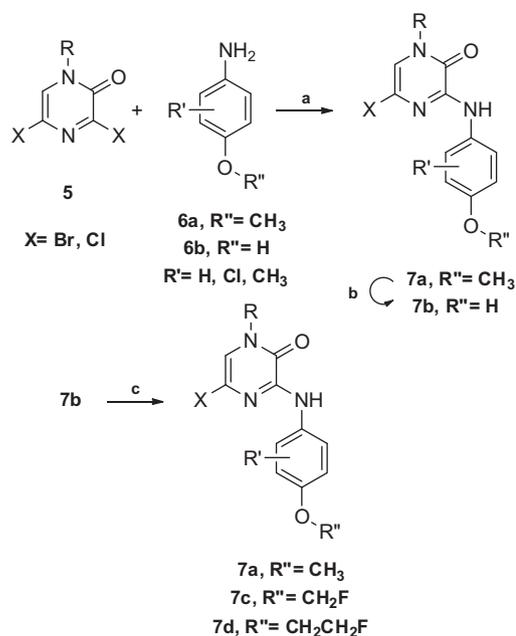
**Scheme 1.** Reagents and conditions: (a) NaHMDS, THF; (b) BBr<sub>3</sub>, CH<sub>2</sub>Cl<sub>2</sub>, -78 °C; (c) CH<sub>3</sub>I or FCH<sub>2</sub>Br or FCH<sub>2</sub>CH<sub>2</sub>Br, KOH, DMSO, 65 °C.
