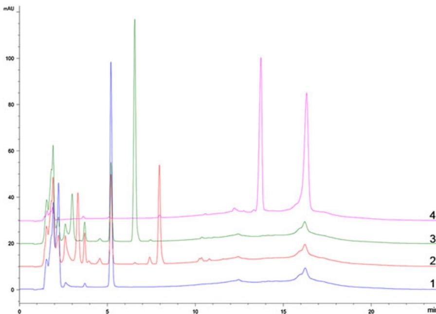
**Fig. 4.** Reversed phase high-performance liquid chromatography measurement of (+)-*O,O*-dibenzoyl-L-tartaric monoesters: hydrolyzed (+)-*O,O*-dibenzoyl-L-tartaric anhydride (1) and respective monoesters of quinine (2), quinidine (3), and *rac*-*N*-allyl-mefloquine (4).
