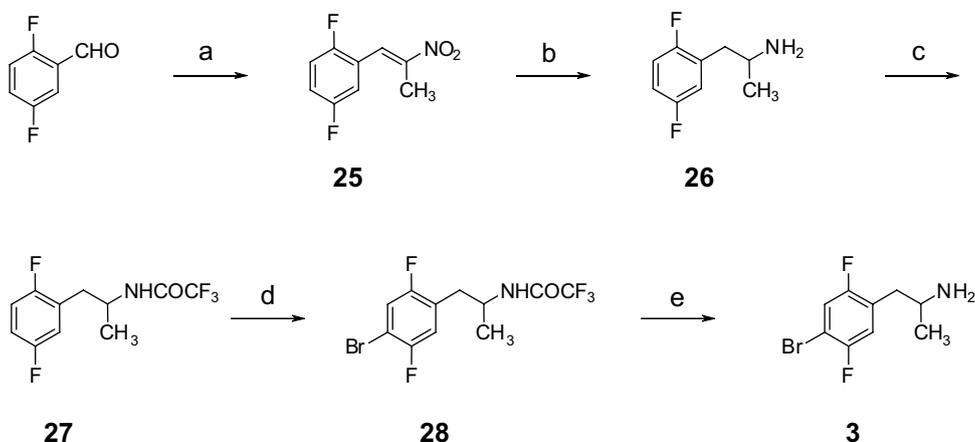
**Scheme 1.** Synthesis of fluorinated phenethylamine derivative **3**.<sup>a</sup> Reagents and conditions: (a) EtNO<sub>2</sub>, *c*-hexNH<sub>2</sub>, HOAc, 91%; (b) NaBH<sub>4</sub>, BF<sub>3</sub>·OEt, 77%; (c) (CF<sub>3</sub>CO)<sub>2</sub>O, Et<sub>3</sub>N, 66%; (d) Br<sub>2</sub>, Ag<sub>2</sub>SO<sub>4</sub>, H<sub>2</sub>SO<sub>4</sub>, 44%; (e) NaOH, H<sub>2</sub>O/MeOH, 50%.
