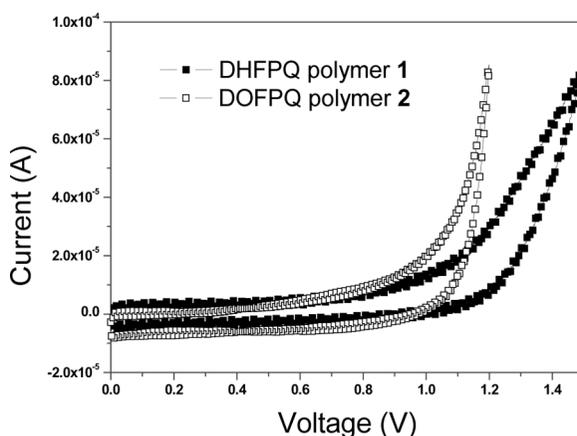
**FIGURE 2** Cyclic voltammetry of oxidation of a 100-nano-thick polymer **1** and **2** film spin-coated over an ITO electrode with 0.1 M  $\text{Bu}_4\text{NClO}_4$  in DMF as the supporting electrolyte. Scan rate 50 mV/s.
