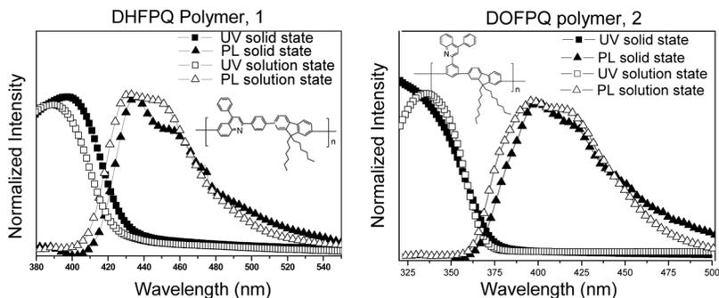
**FIGURE 1** (a) Normalized optical absorption and PL emission spectra of  $10^{-5}$  M solutions in  $\text{CHCl}_3$  and thin films of copolymer **1** and **2**. The excitation wavelength was 350 nm. Normalized PL emission spectra of the polymer thin films annealed at  $100^\circ\text{C}$  in air.
