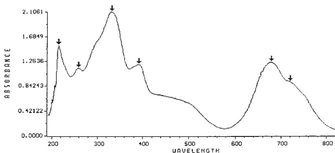
Fig. 2. The UV-vis absorption spectrum of Pc 19.
