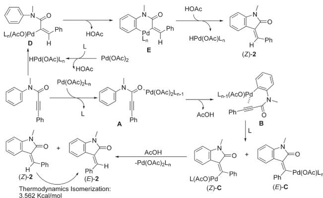
the desired products (**Z**)-**2** and/or (**E**)-**2**. The products (**Z**)-**2** can be converted to (**E**)-**2** under thermodynamics control. Another route cannot be ruled out: HPd(OAc)L<sub>n</sub> is generated *in situ* from the reaction of Pd(OAc)<sub>2</sub> with ligand,<sup>11</sup> followed by *cis*-hydropalladation of alkyne to afford intermediate **D**. Sequential C–H activation/reductive elimination of intermediate **D** gives the product (**Z**)-**2**.
