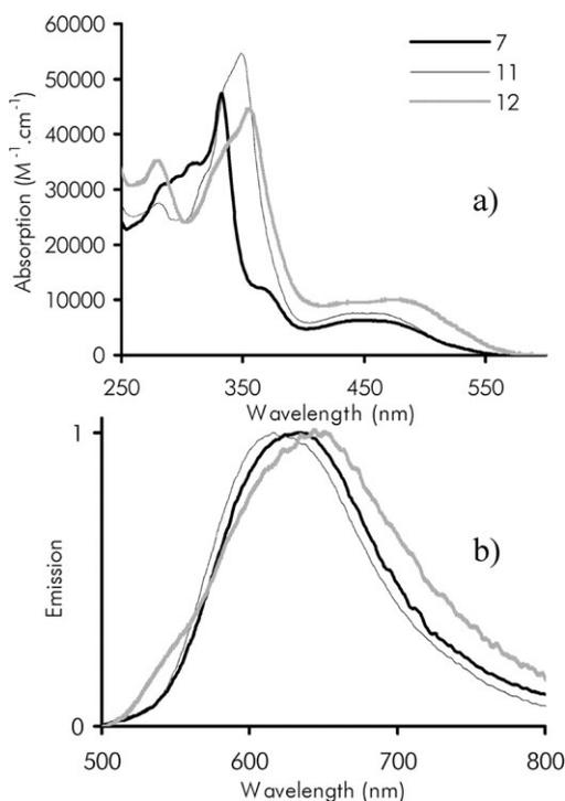
**Fig. 3** (a) Overlay of absorption spectra recorded for the fluorene series in dichloromethane solution at rt. (b) Phosphorescence spectra measured at rt, in dichloromethane in air, with an excitation wavelength of 446 nm for **7**, 444 nm for **11** and 475 nm for complex **12**.
