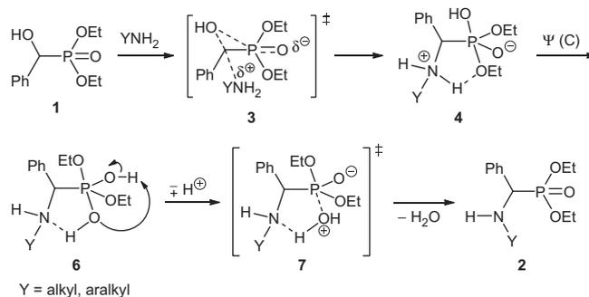
**Scheme 2.** Mechanism for the substitution of diethyl  $\alpha$ -hydroxy-benzylphosphonate by amines supported by B3LYP/6-31G(d,p) calculations.
