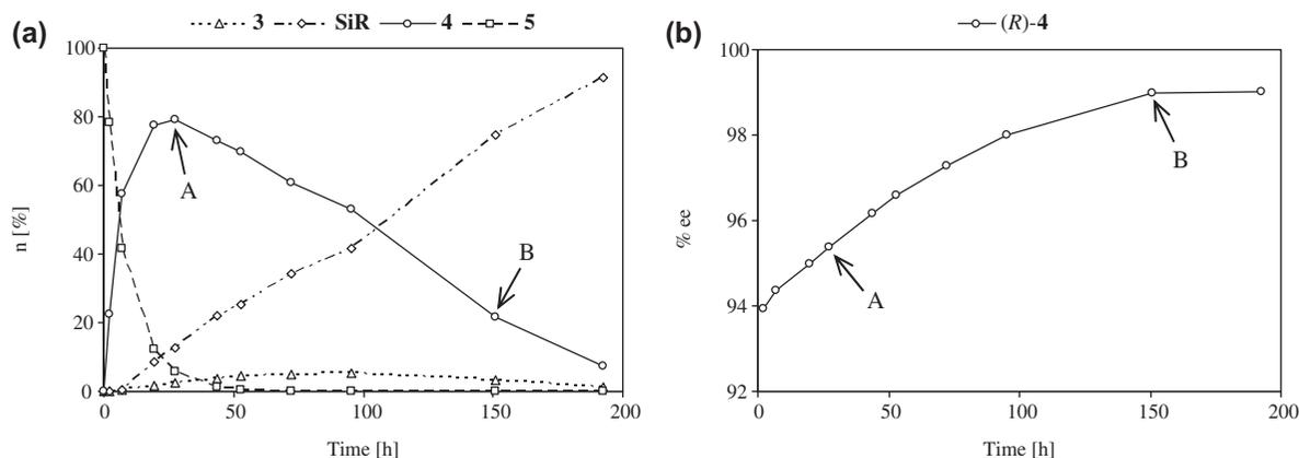
Figure 4. Reaction course of the hydrolysis of diacetate **5** carried out with lipase from *B. cepacia*; a: Amount of compounds **3**, SiR = Me<sub>2</sub>PhSiOH, **4** and **5** (n [%]); b: Enantiomeric excess of (*R*)-**4** [% ee]; Sample A (27.3 h): 79.2% of **4**, 95.4% ee of (*R*)-**4**; Sample B (150.8 h): 21.8% of **4**, 99.0% ee of (*R*)-**4**.
