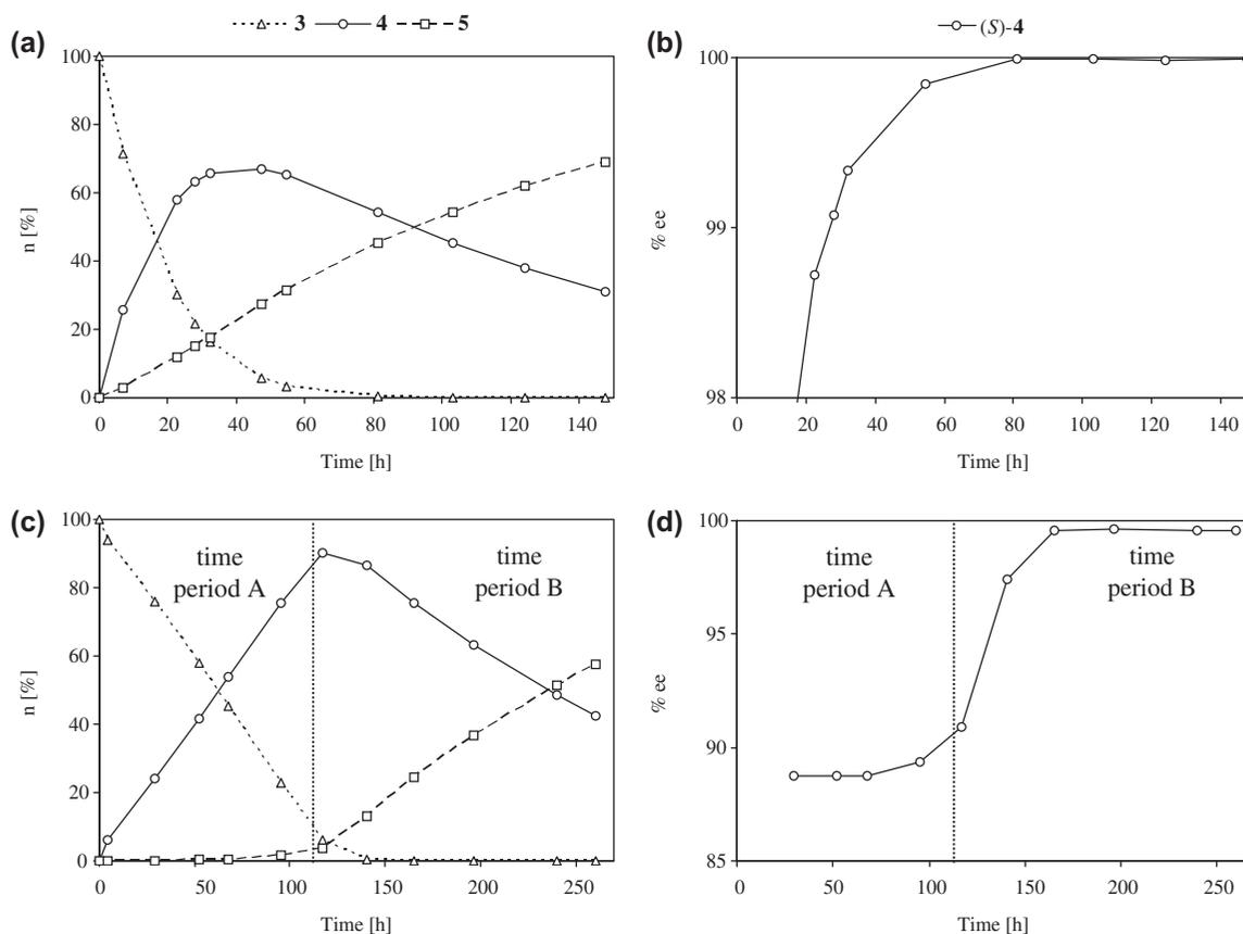
Figure 3. Reaction course of the acetylation of diol **3** carried out with lipase from *B. cepacia* (a, b) and with lipase from *M. miehei* (c, d); a, c: Amount of compounds **3**, **4** and **5** (n [%]); b, d: Enantiomeric excess of (*S*)-**4** [% ee].
