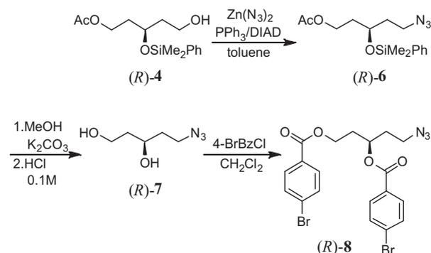
Figure 5. In order to determine the absolute configuration of (*R*)-**4** by CD-spectroscopy, (*R*)-**8** was produced as described in literature for the (*S*)-configured enantiomer (Köhler & Wünsch 2006).
