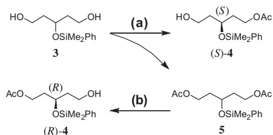
Figure 2. Reaction scheme of the lipase catalysed reactions. (a) Acetylation of diol **3** using isopropenyl acetate as acylating agent in *tert*-butyl methyl ether led to monoacetate (*S*)-**4** in enantiomeric excess and diacetate **5** as a side product. (b) Hydrolysis of diacetate **5** in aqueous buffer solution gave (*R*)-**4** in enantiomeric excess.
