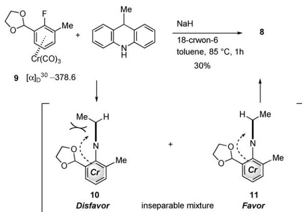
**Scheme 5** Synthesis of complex **8** by nucleophilic substitution and chromium tricarbonyl migration reaction in one pot.
