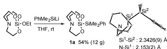
Figure 1. Synthesis and ORTEP drawing of silylsilatrane **1a**. Thermal ellipsoids represent 50% probability.
