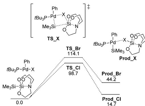
Figure 2. Energy profile of the transmetalation reaction obtained by DFT calculations at the M06/6-311G\*\*+ECP(Pd,P,Si,Cl,Br) level. Energies are in  $\text{kJ mol}^{-1}$ .
