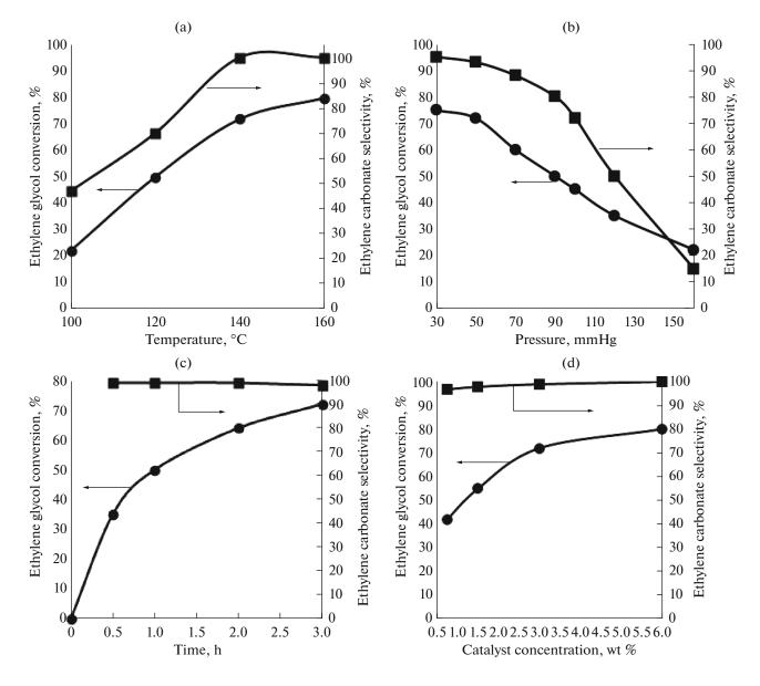
Fig. 1. Effect of cyclocondensation reaction conditions on ethylene glycol conversion and EC selectivity in the presence of  $Co(acac)_3$ : effect of (a) temperature, (b) pressure, (c) contact time, and (d) catalyst concentration on ethylene glycol conversion and EC selectivity.
