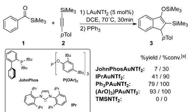
**Scheme 1.** Gold(I)-catalyzed formation of indene **3**.<sup>[a]</sup> Yields and conversions were determined by NMR spectroscopy with 1,3,5-trimethoxybenzene as the internal standard.
