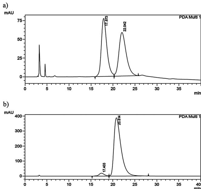
**Fig. 3.** Chiral HPLC trace of (1*S*,2*R*)-Dimethyl 1,2-diphenylcyclopropylphosphonate (**5**) (a) prepared using Rh<sub>2</sub>(OAc)<sub>4</sub> (Racemic sample) (b) prepared using Rh<sub>2</sub>(S-1,2-NTTL)<sub>4</sub>. Chromatographic conditions: Chiralcel OJ column, 2% 2-propanol in *n*-hexane (*v/v*%), 1 mL/min., 220 nm.
