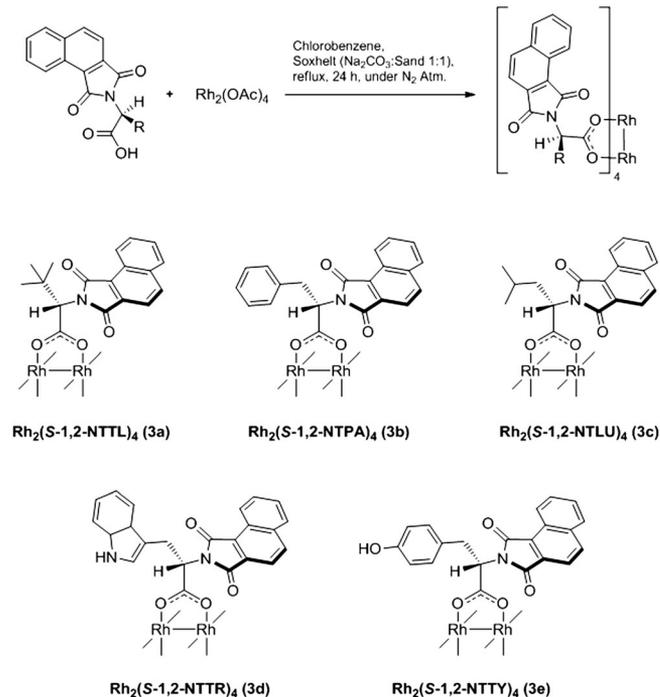
Scheme 3. Preparation and structure of new catalysts.
