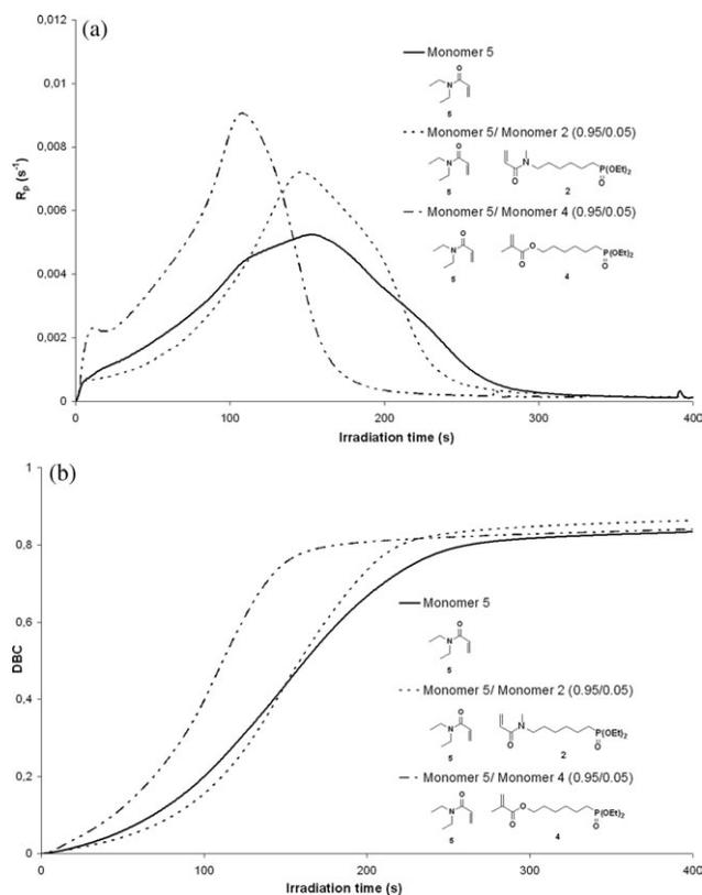
**FIGURE 2** Fractional conversion rate (a) and fractional conversion (b) of double bonds versus irradiation time for the homopolymerization of Monomer 5 and its copolymerization with Monomers 2 or 4.
