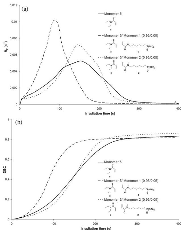
**FIGURE 3** Fractional conversion rate (a) and fractional conversion (b) of double bonds versus irradiation time for the homopolymerization of Monomer 5 and its copolymerization with Monomers 1 and 2.
