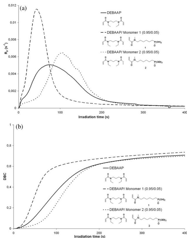
**FIGURE 5** Fractional conversion rate (a) and fractional conversion (b) of double bonds versus irradiation time for the homopolymerization of DEBAAP and its copolymerization with Monomers 1 and 2.
