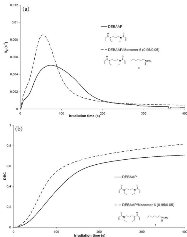
**FIGURE 7** Fractional conversion rate (a) and fractional conversion (b) of double bonds versus irradiation time for the homopolymerization of DEBAAP and its copolymerization with species **6**.
