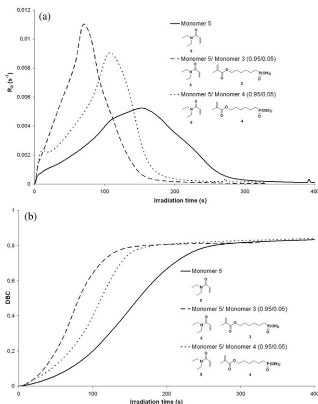
**FIGURE 4** Fractional conversion rate (a) and fractional conversion (b) of double bonds versus irradiation time for the homopolymerization of Monomer 5 and its copolymerization with Monomers 3 and 4.
