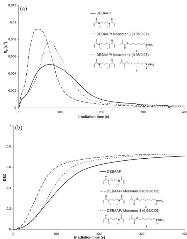
**FIGURE 6** Fractional conversion rate (a) and fractional conversion (b) of double bonds versus irradiation time for the homopolymerization of DEBAAP and its copolymerization with Monomers **3** and **4**.
