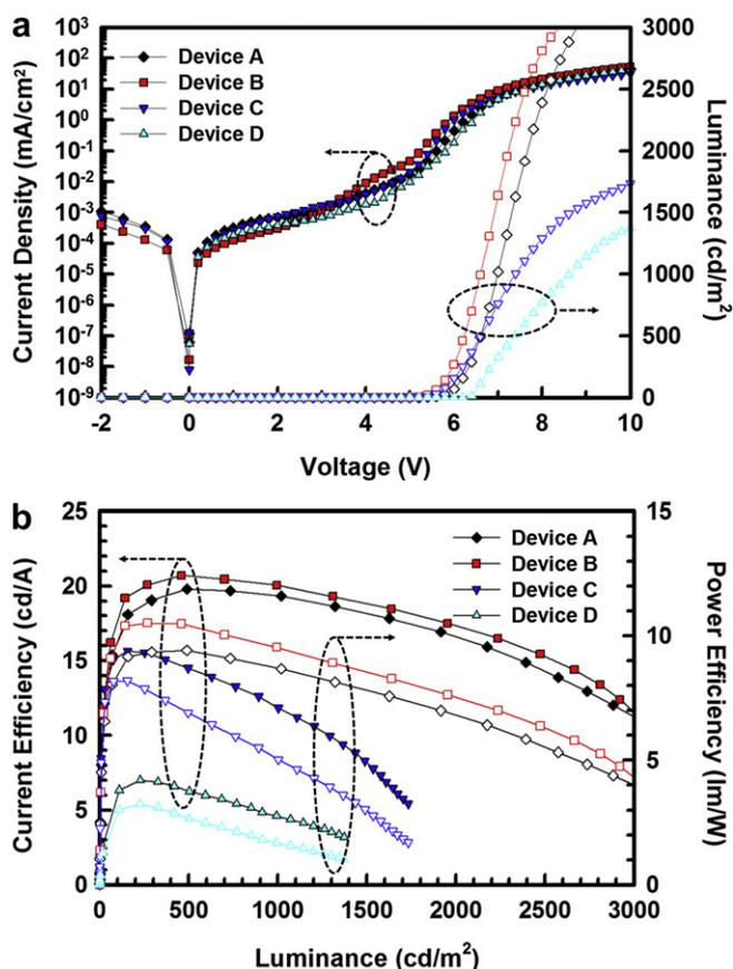
**Fig. 6.** a)  $J-V-L$  characteristics of fabricated blue PHOLEDs. b) Luminance vs current efficiency and power efficiency characteristics of fabricated blue PHOLEDs. (For interpretation of the references to colour in this figure legend, the reader is referred to the web version of this article.)
