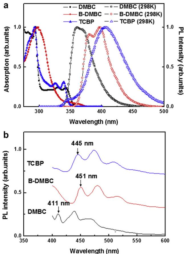
Fig. 2. (a) UV–visible absorption and photoluminescence spectra (at 298 K), (b) photoluminescence spectra (at 77 K) of three host materials in 2-methyl tetrahydrofuran.
