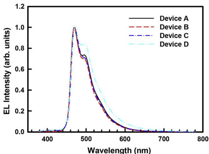
Fig. 8. EL spectra at a brightness of 1000 cd/m<sup>2</sup> of different fabricated blue PHOLEDs. (For interpretation of the references to colour in this figure legend, the reader is referred to the web version of this article.)
