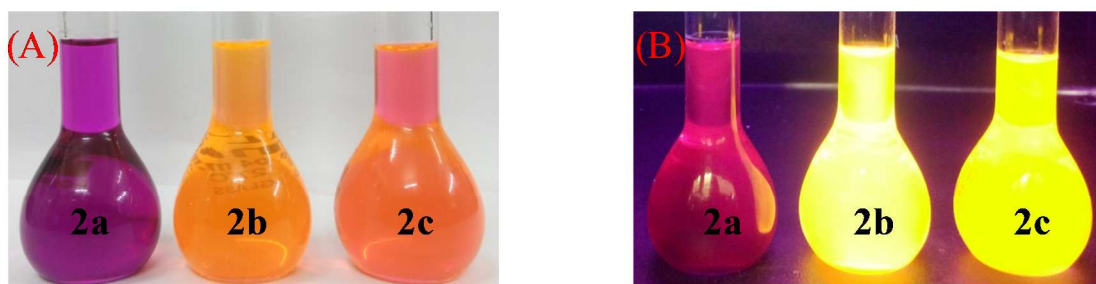
Fig. 2 The BODIPYs 2a–2c in toluene at concentration of 10^{-4} M in day light (A) and in UV light (B).
