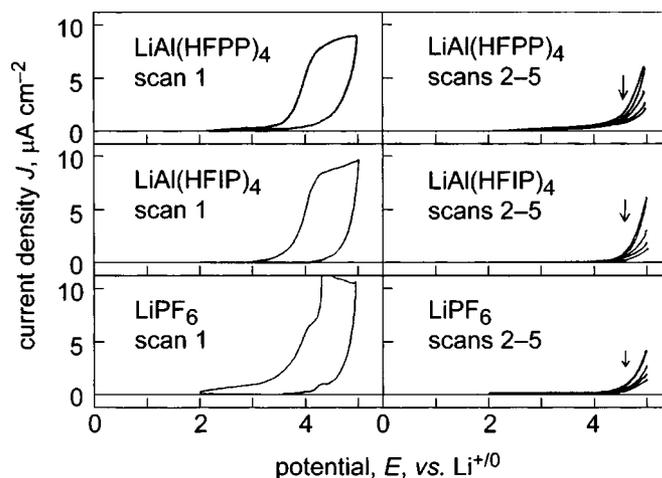
**Figure 7.** CVs of 0.3 M propylene carbonate solutions of LiAl(HFIP)<sub>4</sub>, LiAl(HFPP)<sub>4</sub>, and LiPF<sub>6</sub>. Conditions: aluminum working electrode, lithium foil counter and reference electrodes, 10 mV s<sup>-1</sup>.
