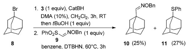
Scheme 7. Oximation of adamantyl bromide with silylboranes involving a 1,5-hydrogen transfer process. Bn = benzyl.
