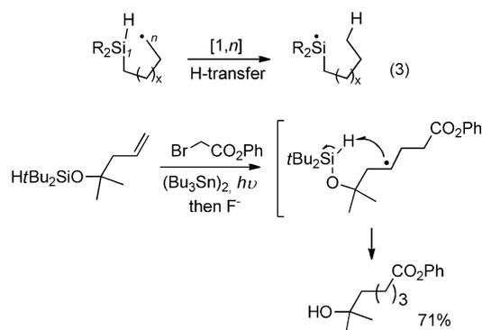
Scheme 3. 1,5-Hydrogen transfer from Si to C.
