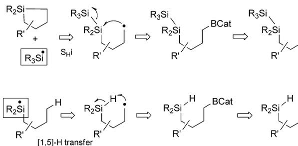
Scheme 4. Silylboranes producing silyl radicals through  $\text{S}_{\text{H}}\text{i}$  and 1,5-hydrogen transfer processes. Cat = catechol.
