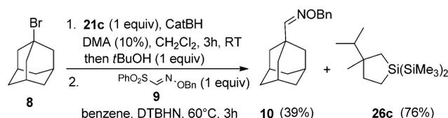
Scheme 14. Oximation of adamantyl bromide using silylboranes involving an  $S_{\text{H}}\text{i}$  process.
