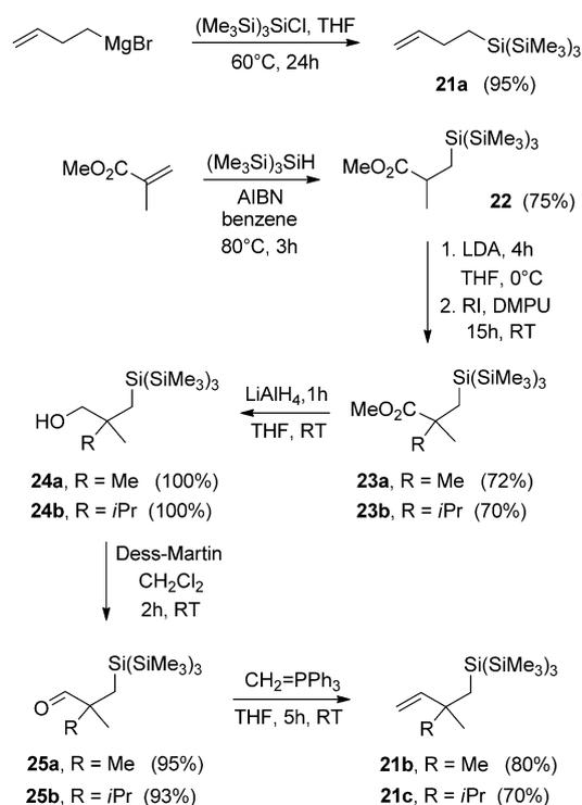
Scheme 12. Synthesis of  $S_{\text{H}1}$  precursors **21a–c**. LDA = lithium diisopropyl amide, DMPU = 1,3-dimethyl-3,4,5,6-tetrahydro-2(1*H*)-pyrimidinone.
