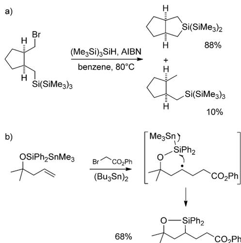
Scheme 2. Intramolecular homolytic substitution at a silicon center. AIBN = azobisisobutyronitrile.
