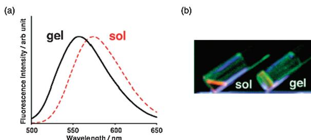
**Figure 4.** (a) Fluorescence spectra of **1** ( $[1] = 4.0$  mM, solvent: 1-decanol,  $\lambda_{\text{ex}} = 350$  nm, optical path length: 1.0 mm, temperature: 25 °C.), (b) the image of **1** + 1-decanol sol and gel.
