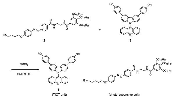
**Figure 2.** Synthesis and chemical structure of compound **1**: CsCO<sub>3</sub> (16 equiv), DMF/THF (4:3, v/v), 100 °C, 24 h, 65%.
