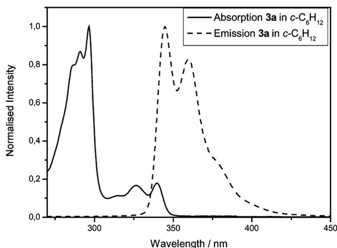
Figure 5. Absorption and emission spectra of **3a**.
