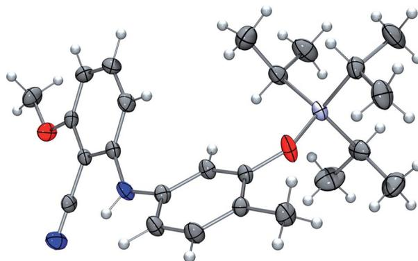
Figure 4. Molecular structure of diarylamine **25** in the crystal. ORTEP plot showing thermal ellipsoids at 50% probability level.
