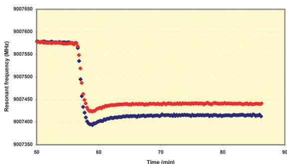
**Fig. 2** TSM resonant frequency responses to 10% goat serum injection for (bottom – blue) bare and (top – red) HS-MEG-OH adlayer-derivatized gold surfaces. For comparison purposes, injection times ( $t \sim 56$  min) and initial resonant frequencies have been normalized.
