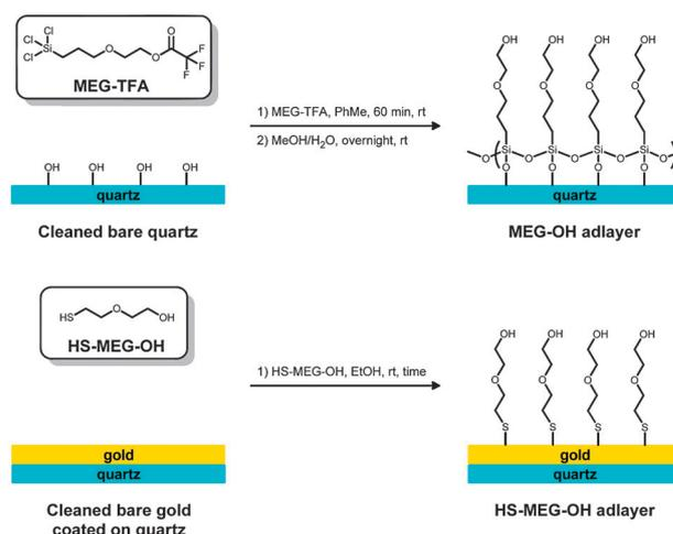
**Fig. 1** Surface modification of (top) hydroxylated quartz and (bottom) gold metal with MEG-OH adlayers.
