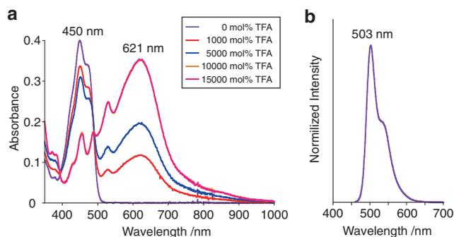
**Figure 4.** (a) UV-vis-NIR spectra of **1b** (0.05 mM) and **1b** with 1000, 5000, 10000, and 15000 mol% CF<sub>3</sub>CO<sub>2</sub>H in CH<sub>2</sub>Cl<sub>2</sub>. (b) Emission spectrum of **1b** (0.02 mM) in CH<sub>2</sub>Cl<sub>2</sub> (excited at 450 nm).
