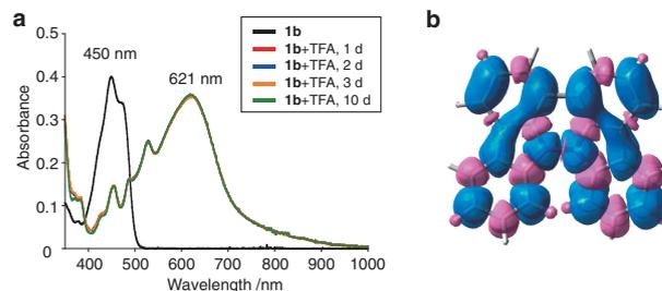
**Figure 7.** (a) UV-vis-NIR spectra of **1b** (0.05 mM) with 10000 mol%  $\text{CF}_3\text{CO}_2\text{H}$  in  $\text{CH}_2\text{Cl}_2$  after 1, 2, 3, and 10 d at 20 °C under air. (b) Calculated spin density distribution of  $\text{BC}^{+\cdot}$  [U $\omega$ B97XD/6-31G(d)]. Blue and pink colors indicate the positive and negative spin density, respectively.
