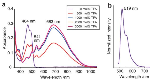
**Figure 6.** UV-vis-NIR spectra of **1c** (0.03 mM) with 0, 500, 1000, 2000, and 3000 mol%  $\text{CF}_3\text{CO}_2\text{H}$  in  $\text{CH}_2\text{Cl}_2$ . (b) Emission spectrum of **1c** (0.02 mM) in  $\text{CH}_2\text{Cl}_2$  (excited at 464 nm).
