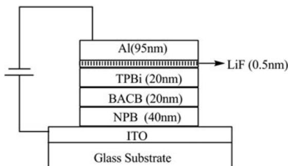
FIGURE 6 The structure of the EL device
