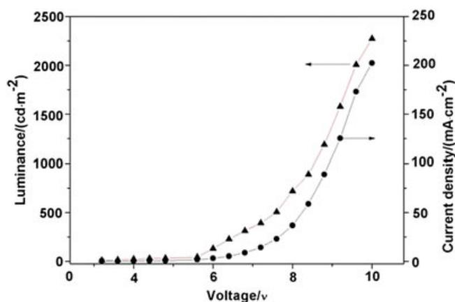
FIGURE 8 The luminance-voltage-current density curves of the device
