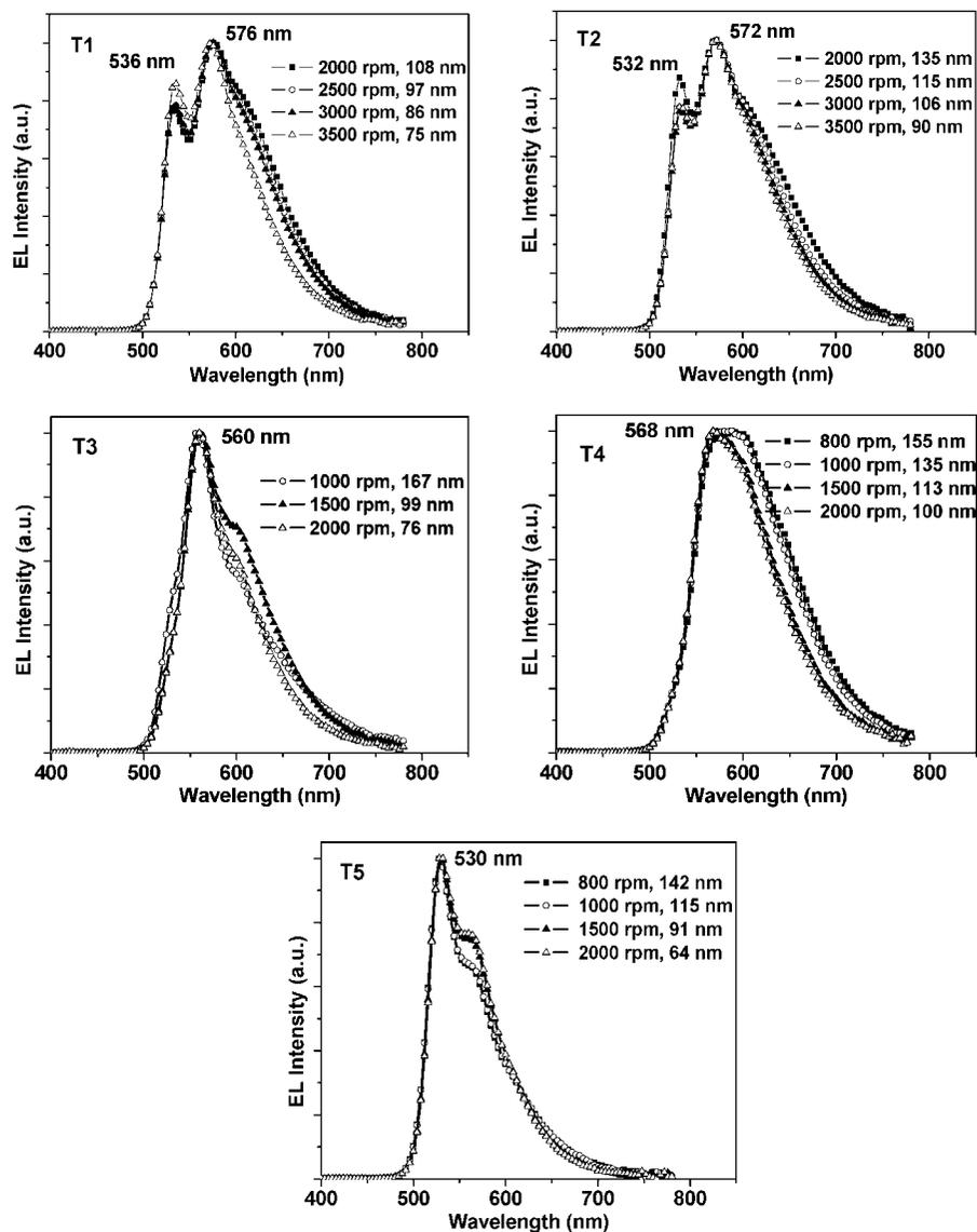
**FIGURE 6.** EL spectra of dendrimer devices with a configuration of ITO/PEDOT/T1–T5/Cs<sub>2</sub>CO<sub>3</sub>/Al.
