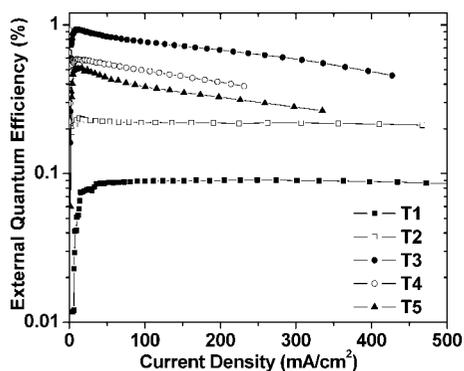
FIGURE 8. External quantum efficiency curves of the most efficient devices based on T1–T5.
