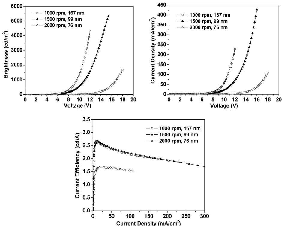
FIGURE 7. *J-V-L* characteristics and current efficiency curves of T3-based devices with a configuration of ITO/PEDOT/T3/Cs<sub>2</sub>CO<sub>3</sub>/Al.
