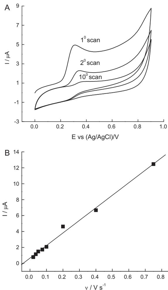
Fig. 3. Cyclic voltammetry of 0.1 mmol L<sup>-1</sup> MGN in phosphate buffer pH 7.0 on GC electrode. Scan rate 100 mV s<sup>-1</sup>.
