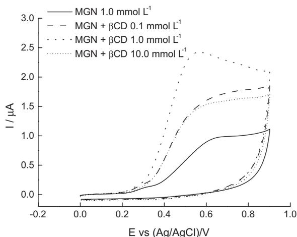
**Fig. 4.** Cyclic voltammograms recorded in  $\text{Na}_2\text{SO}_4$   $0.2 \text{ mol L}^{-1}$  of MGN ( $1.0 \text{ mmol L}^{-1}$ ), pH 7.0, in the presence of free  $\beta$ -CD concentration.
