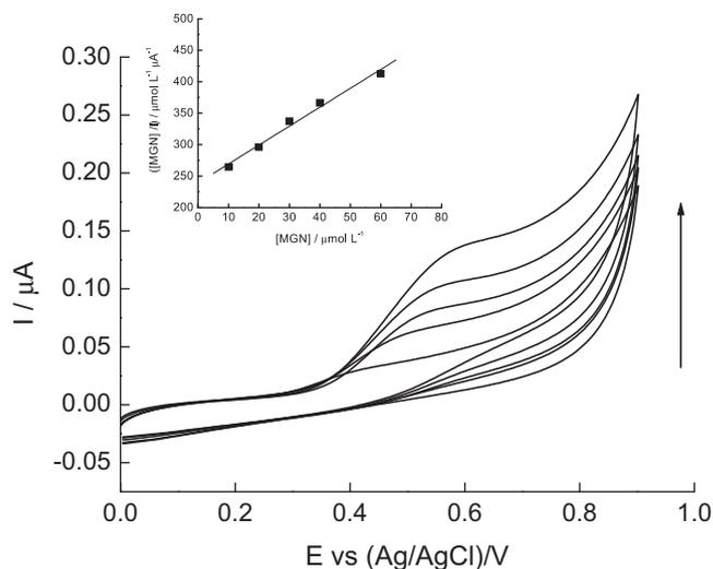
**Fig. 6.** Cyclic voltammograms recorded in  $0.2 \text{ mol L}^{-1}$   $\text{Na}_2\text{SO}_4$  solution at different concentrations of MGN ( $5 \mu\text{mol L}^{-1}$  up to  $60 \mu\text{mol L}^{-1}$ ). Inset: Determination of the equilibrium constant of the MGN: $\beta$ -CD.
