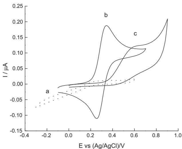
**Fig. 5.** Voltammetric response of  $1.0 \times 10^{-3} \text{ mol L}^{-1}$   $\text{K}_3[\text{Fe}(\text{CN})_6]$  (curve a),  $1.0 \times 10^{-4} \text{ mol L}^{-1}$   $\text{Fc-CO}_2\text{H}$  (curve b),  $6.0 \times 10^{-5} \text{ mol L}^{-1}$  MGN (curve c) on SAM  $\beta$ -CD modified electrode in  $0.2 \text{ mol L}^{-1}$   $\text{Na}_2\text{SO}_4$ . Scan rate =  $10 \text{ mV s}^{-1}$ .
