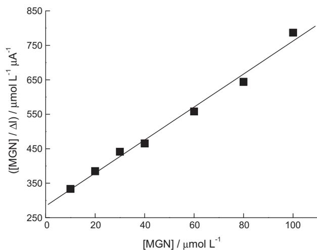
**Fig. 7.** Plot of  $[MGN]/\Delta I$  (difference between the peak current of the redox processes of Fc-CO<sub>2</sub>H in the presence and absence of MGN) vs.  $[MGN]$  on CDSH/MUA modified electrode at Na<sub>2</sub>SO<sub>4</sub> 0.1 mol L<sup>-1</sup>.
