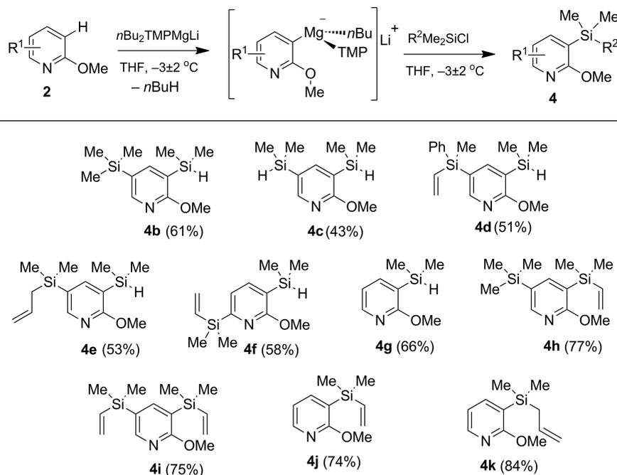
Scheme 3. 3-Silyl-functionalised 2-methoxypyridines obtained by *ortho*-metallation using the novel nBu<sub>2</sub>TMPMg Li.
