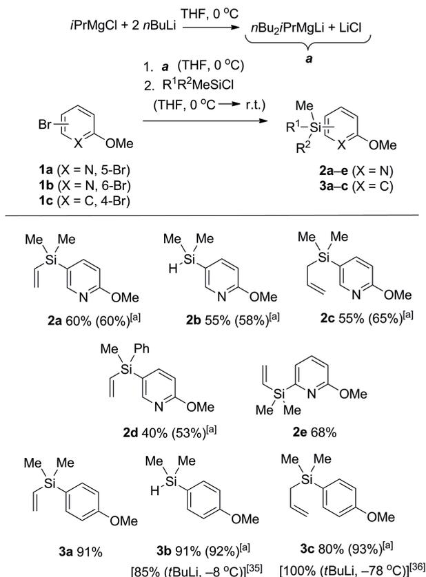
Scheme 2. Synthesis of 5-silyl-functionalised 2-methoxypyridines **2a–2e** and 4-silyl-functionalised anisoles **3a–3c**. [a] Yields estimated by  $^1\text{H}$  NMR spectroscopy using an internal reference are given in the parentheses.
