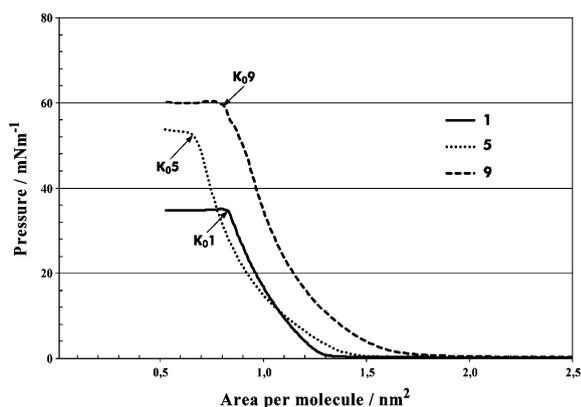
**Fig. 3** Isotherms ( $\pi$ - $A$ ) of the amphiphiles **1**, **5** and **9**, featuring different degrees of branching of the hydrophilic segment: **1** (unbranched), **5** (first generation branching), **9** (second generation branching).
