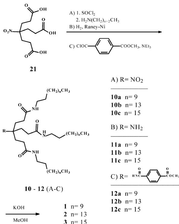
Scheme 5 Synthesis of the first generation monodendritic amphiphiles 1–3, involving an aromatic spacer unit.
