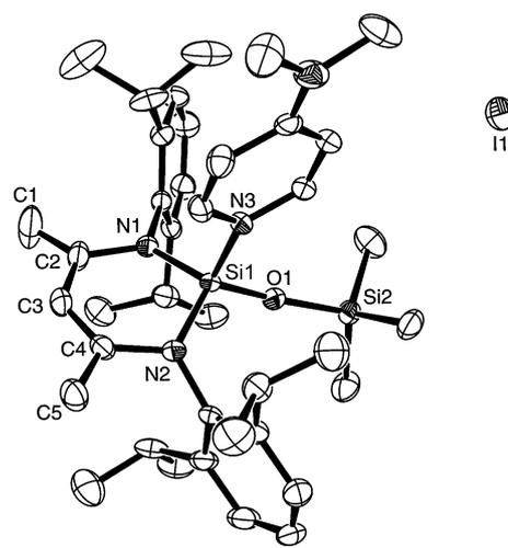
Figure 4. Molecular structure of **5**. Thermal ellipsoids are drawn at the 50% probability level. Hydrogen atoms and THF molecules are omitted for clarity. The iodide anion and solvent THF molecules are in disorder. Selected bond lengths [Å] and angles [°]: Si1–O1 1.582(3), Si2–O1 1.662(3), Si1–N1 1.709(3), Si1–N2 1.717(3), Si1–N3 1.811(3); Si1–O1–Si2 165.1(2), N2–Si1–N3 106.8(2), N1–Si1–N3 109.4(2), N1–Si1–N2 106.0(2), O1–Si1–N1 114.4(2), O1–Si1–N2 115.3(2), O1–Si1–N3 104.6(2).
