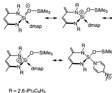
Scheme 5. Resonance structures of the  $[\text{LSi}(\text{dmap})=\text{O}-\text{SiMe}_3]^+$  cation in **3** and **5**.
