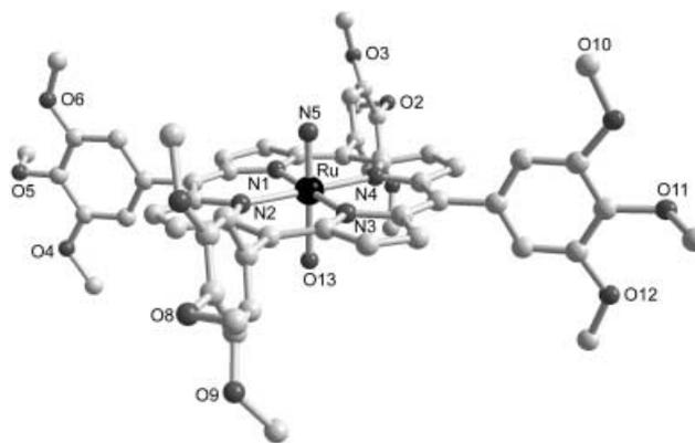
**Figure 1.** Molecular structure of **1b** determined by X-ray crystallography (hydrogen atoms are not shown). Selected bond lengths [Å] and bond angles [°]: Ru–N1 2.046(6), Ru–N2 2.086(6), Ru–N3 2.001(6), Ru–N4 2.026(7), Ru–N5 1.656(5), Ru–O13 2.086(7); N1–Ru–N2 92.7(2), N2–Ru–N3 88.5(2), N3–Ru–N4 88.5(3), N4–Ru–N1 90.3(3), N5–Ru–O13 177.8(3).
