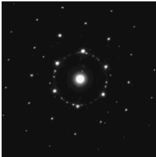
**Fig. 9.** Selective electron diffraction pattern of  $\text{Pb}(\text{Zr}_{0.52}\text{Ti}_{0.48})\text{O}_3$  (PZT) microtubes from the area in Fig. 8(c). The single crystalline pattern originates from the large single crystals of PZT, whereas the polycrystalline ring is from the smaller pyrochlore phase.
