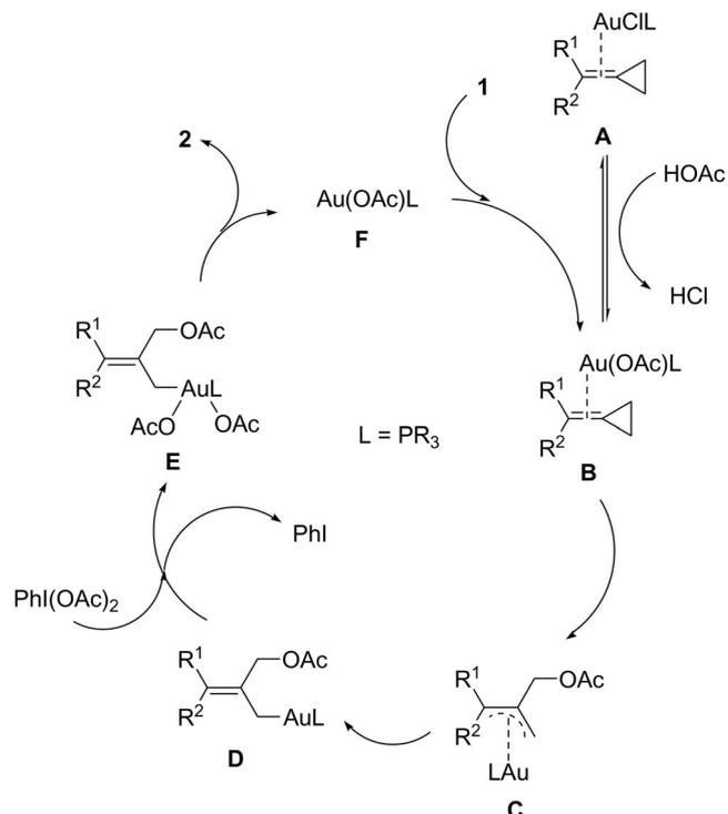
Scheme 4. A plausible reaction mechanism.
