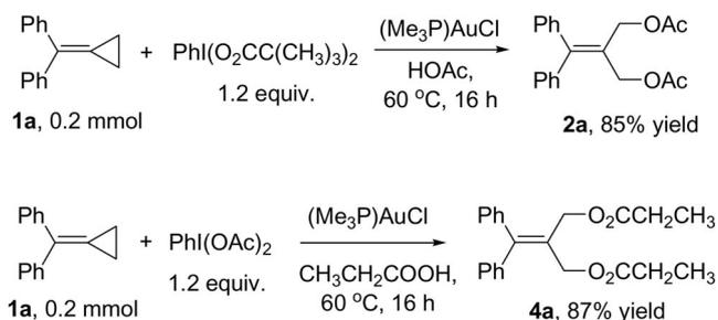
Scheme 3. Control experiments of MCP **1a** with iodosobenzene dicarboxylates under the standard conditions.
