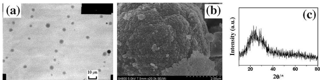
**Fig. 1** As-synthesized DCNs: (a) TEM image (scale bar = 10  $\mu\text{m}$ ); (b) SEM image (scale bar = 2  $\mu\text{m}$ ). (c) The XRD diffractogram of the DCNs.
