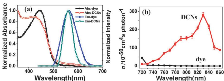
**Fig. 2** (a) Normalized UV-vis absorption and PL spectra of **dye** and **DCNs** in DMF. The fluorescence was excited at 445 nm for the **dye** and 431 nm for **DCNs**, respectively; (b) TPA cross section of **dye** and **DCNs** in DMF *versus* excitation wavelengths from 720 nm to 860 nm in DMF.
