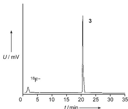
**Figure 3.** Top: synthesis of **3** using **4** and  $^{18}\text{F}^-/\text{Kryptofix 2.2.2./K}^+$ ; Bottom: radio-HPLC chromatogram of the crude reaction mix of **4** (1  $\mu\text{g}$  (4.1 nM)) with  $^{18}\text{F}^-/\text{Kryptofix 2.2.2./K}^+$  complex (1 GBq) in  $\text{CH}_3\text{CN}$  (100  $\mu\text{L}$ ) after 15 min reaction time at room temperature.
