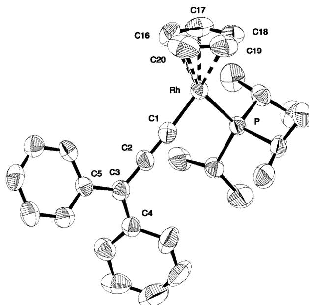
**Figure 1.** Molecular diagram of compound **3**. Selected bond distances (Å) and angles (deg): Rh–P, 2.2700(15); Rh–C1, 1.880(6); Rh–C16, 2.237(6); Rh–C17, 2.253(7); Rh–C18, 2.242(6); Rh–C19, 2.231(7); Rh–C20, 2.198(7); C1–C2, 1.255(7); C2–C3, 1.350(7); C3–C4, 1.466(8); C3–C5, 1.465(7); P–Rh–C1, 89.48(17); Rh–C1–C2, 177.1(5); C1–C2–C3, 176.5(6); C2–C3–C4, 119.3(5); C2–C3–C5, 120.2(5); C4–C3–C5, 120.5(5).
