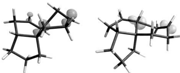
Scheme 23. 6-endo cis - and trans -transition states geometries (spin density: balls).
