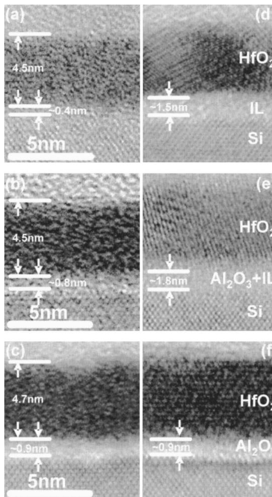
FIG. 3. Cross-sectional HRTEM images of HfO<sub>2</sub>–ultrathin-Al<sub>2</sub>O<sub>3</sub>–Si structures as-deposited [(a)–(c)] and after thermal annealing in N<sub>2</sub> for 10 s at 700 °C; the number of Al<sub>2</sub>O<sub>3</sub> ALD cycles increases from zero to 5 to 10 in the sequences (a)–(c) and (d)–(f). “IL” stands for interfacial layer.
