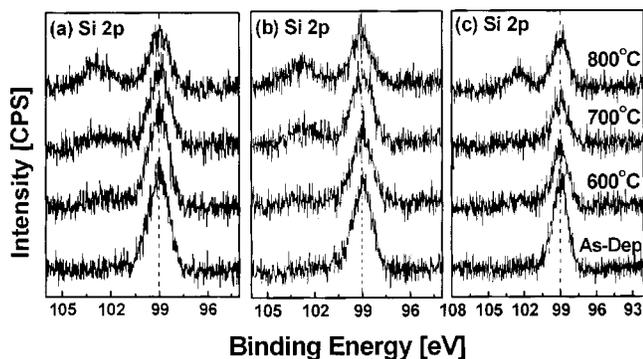
FIG. 2. Si 2*p* XPS data for samples featuring (a) zero, (b) 5, and (c) 10 ALD cycles of Al<sub>2</sub>O<sub>3</sub> between the Si substrate and the HfO<sub>2</sub> overlayer, with annealing temperature as parameter; Si–Si bonding appears at 99 eV, and Si–O at 103 eV.
