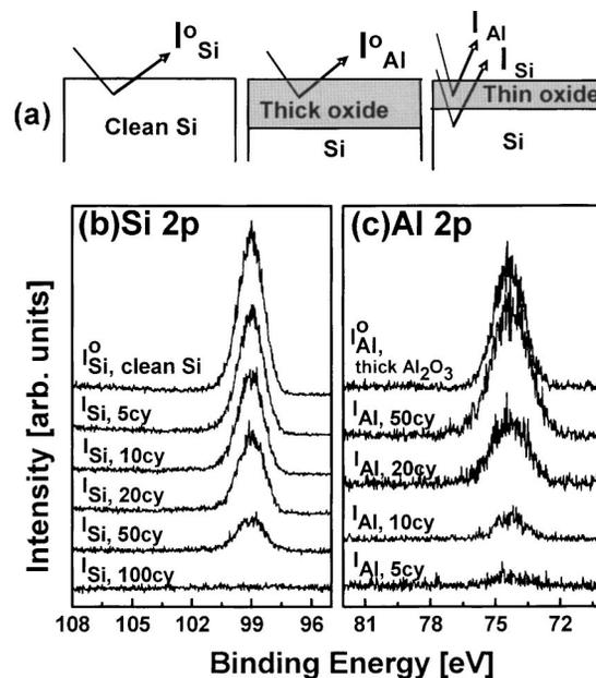
FIG. 1. (a) Schematic illustration of three structures used for Al<sub>2</sub>O<sub>3</sub> thickness determination by XPS: Clean Si substrate, thick Al<sub>2</sub>O<sub>3</sub> film on Si, and thin Al<sub>2</sub>O<sub>3</sub> film on Si (sample of interest); (b) Si 2p and (c) Al 2p XPS data from various thicknesses of as-deposited Al<sub>2</sub>O<sub>3</sub> on Si ("cy" refers to ALD cycles).
