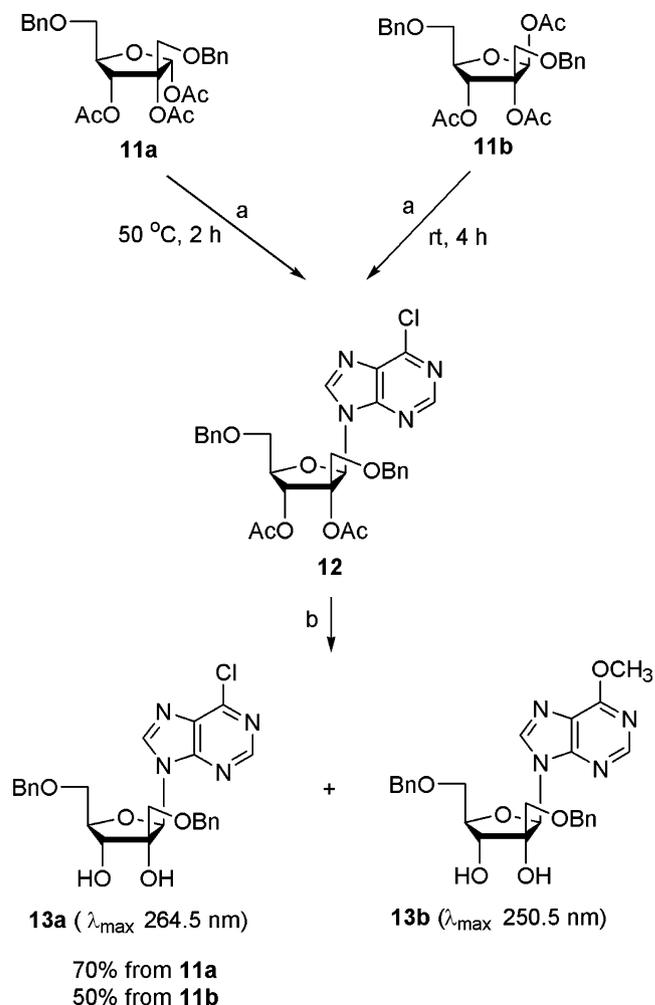
**Scheme 3.** Reagents and conditions: (a) i. 6-chloropurine,  $(\text{NH}_4)_2\text{SO}_4$ , HMDS, 160 °C, overnight; ii. TMSOTf,  $\text{ClCH}_2\text{CH}_2\text{Cl}$ ; (b) NaOMe, MeOH, 1 h.
