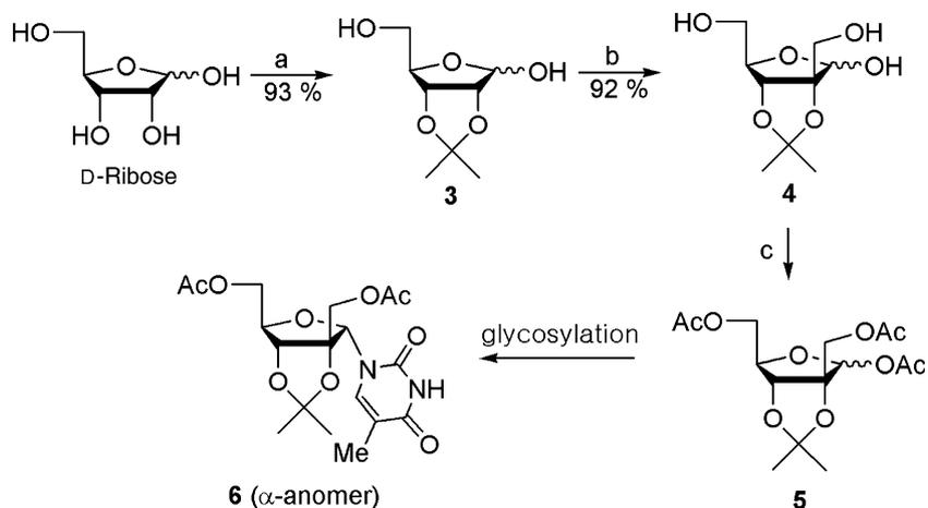
**Scheme 1.** Reagents and conditions: (a) acetone, concd H<sub>2</sub>SO<sub>4</sub>, rt, 2.5 h; (b) CH<sub>2</sub>O, K<sub>2</sub>CO<sub>3</sub>, MeOH, reflux, 4 d; (c) Ac<sub>2</sub>O, DMAP, NEt<sub>3</sub>, rt, 5 h.
