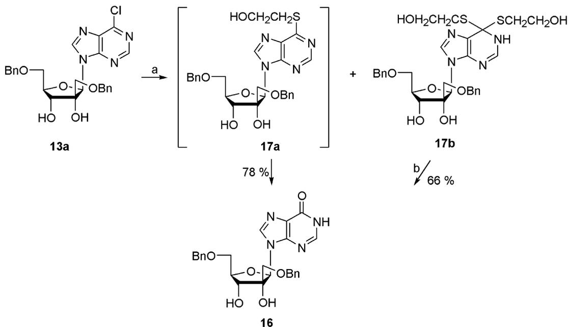
**Scheme 5.** Reagents and conditions: (a) 2-mercaptoethanol,  $\text{NaOMe}$ ,  $\text{MeOH}$ ; (b)  $\text{HgCl}_2$ ,  $\text{AcOH}$ ,  $\text{KOAc}$ , reflux, overnight.
