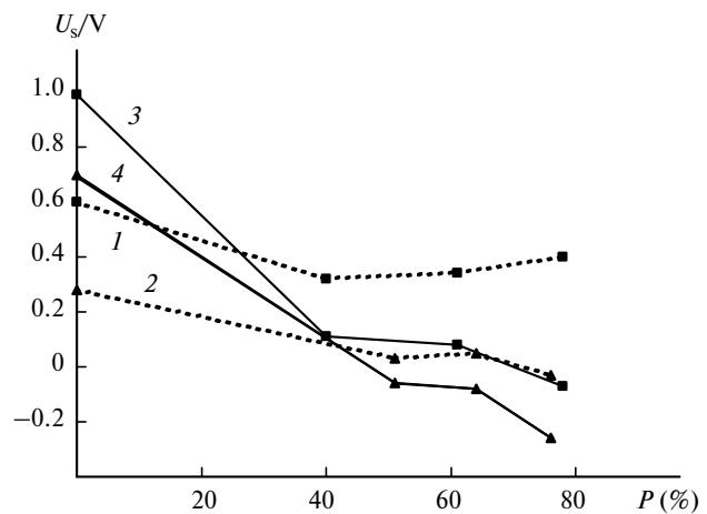
**Fig. 1.** The dependencies of surface potential of PS ( $U_s$ ) on the porosity ( $P$ ) at solubilization extent  $\omega_0 = 5$  for the samples of PS of n-type (1) and p-type (2) and for palladium nanocomposites with PS of n-type (3) and p-type (4).
