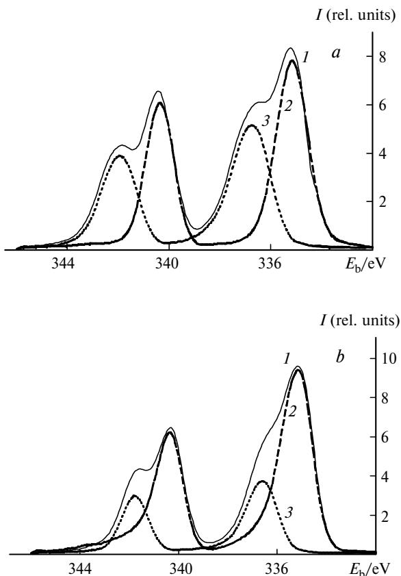
**Fig. 2.** The XPS spectra of Pd ( $3d_{3/2}$  and  $3d_{5/2}$ ) of Pd nanocomposites with PS of n-type (a) and p-type (b) of conductivity: 1 — general view, 2 — Pd<sup>0</sup>, 3 — Pd<sup>2+</sup>.
