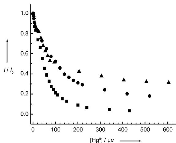
**Figure 4.** Titration of **3** ( $\blacksquare$ ,  $1.0 \times 10^{-5} \text{ M}$ ), **2** ( $\bullet$ ,  $1.0 \times 10^{-5} \text{ M}$ ), and **1** ( $\blacktriangle$ ,  $48 \mu\text{g mL}^{-1}$ ) with  $\text{Hg}^{\text{II}}$  in aqueous solution containing 4%  $\text{CH}_3\text{CN}$  ( $\lambda_{\text{ex}} = 330 \text{ nm}$ ).
