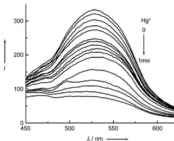
**Figure 1.** Fluorescence spectra of **1** ( $48 \mu\text{g mL}^{-1}$ ) with increasing concentration of  $\text{Hg}^{\text{II}}$  ions in aqueous solution containing 4%  $\text{CH}_3\text{CN}$  ( $\lambda_{\text{ex}} = 330 \text{ nm}$ ).
