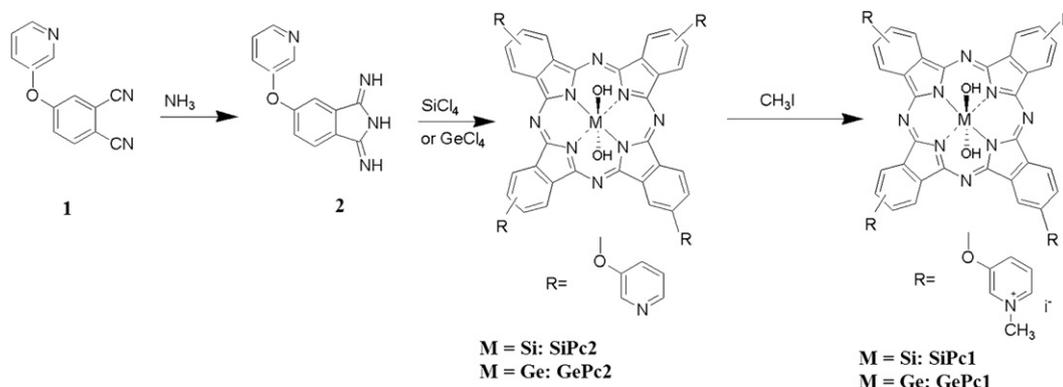
**Scheme 1.** Synthetical pathway of preparation of water-soluble tetra-methylpyridyloxy-substituted Si(IV)-phthalocyanine, SiPc1 and Ge(IV)-phthalocyanine, GePc1.
