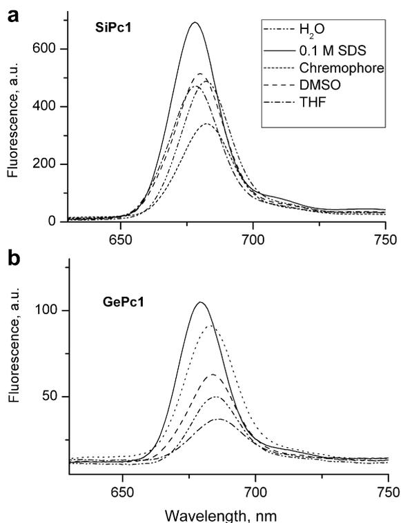
Fig. 2. Fluorescence spectra of SiPc1 (a) and GePc1 (b) in water in comparison to the spectra in presence of detergents and in organic solvents at excitation wavelength,  $\lambda_{exc}$ : 610 nm.
