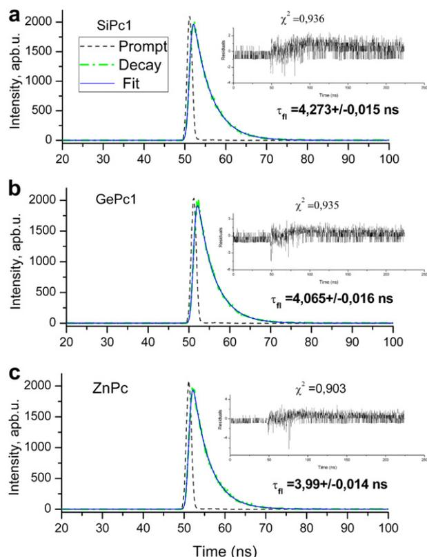
**Fig. 3.** Fluorescence decay of SiPc1 (a) and GePc1 (b), and ZnPc (c), all in DMSO (green dash dot), fit (blue solid line) and instrumental response (dash line) for  $\lambda_{exc} = 365$  nm and fluorescence emission at 683 nm (SiPc1) and 685 nm (GePc1), and 681 nm (ZnPc).
