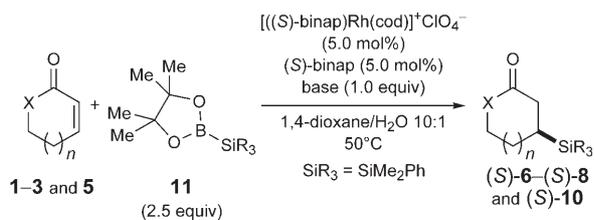
**Scheme 3.** Catalytic asymmetric conjugate silyl transfer (see Tables 2 and 3). binap = 2,2'-bis(diphenylphosphanyl)-1,1'-binaphthyl.
