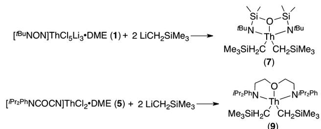
$\text{LiCH}_2\text{SiMe}_3$  to a slurry of **1** in hexanes generated a deep-yellow oil of  $[\text{iBuNON}]\text{Th}(\text{CH}_2\text{SiMe}_3)_2$  (**7**) in 83% yield; this previously reported product was originally synthesized from DME-free  $\{[\text{iBuNON}]\text{ThCl}_2\}_2$ .<sup>65</sup> In this case, despite using the DME-solvated starting material, salt and solvent-free dialkyl products were still obtained.
